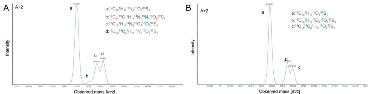
Figure 5. ES-  $\text{MS}^E$  analysis (>200,000 FWHM) precursor and fragment ion spectra obtained for coeluting I) [desmethyl naproxen sulfate -  $\text{H}^-$ ] and II) [carbamazepine-o-sulfate -  $\text{H}^-$ ]. III) (A) carbamazepine-o-sulphate $^-$  and (B) desmethyl naproxen sulfate confirmatory A+2 fine isotope structure obtained using 10 Hz UPLC MRT ES-.
