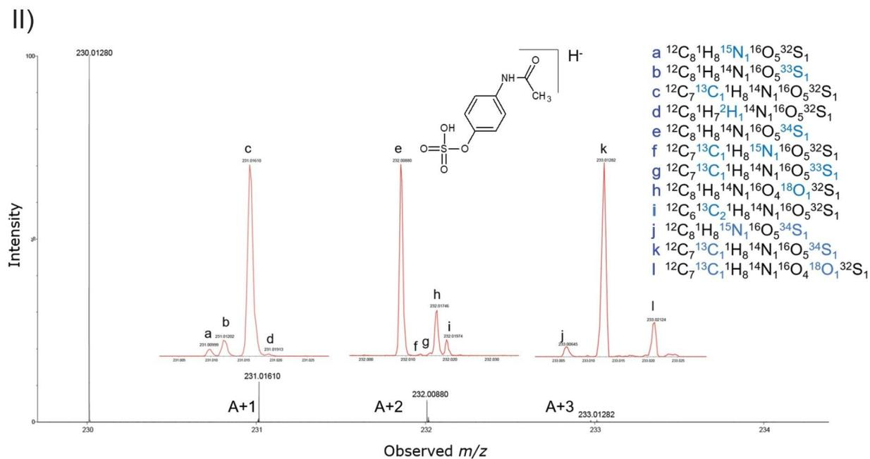
Figure 3. I) 10 Hz UPLC MRT ES- precursor fine isotope spectrum obtained for [acetaminophen sulfate -H]<sup>-</sup> 200,000 FWHM. II) 10 Hz UPLC MRT ES- precursor fine isotope spectrum obtained for [acetaminophen sulfate -H]<sup>-</sup> 300,000 FWHM.
