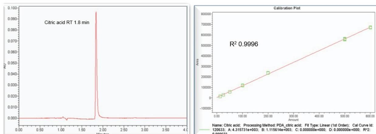
Figure 1. Chromatographic performance and solvent standard calibration curve of citric acid using ACQUITY Premier Column and LC-PDA method. The concentration of the standard is 200 ppm and observed at 210 nm channel on PDA.
